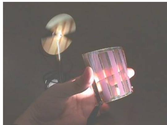
*Konarka's flexible solar cell powers this spinning fan, providing low-cost power from light*
